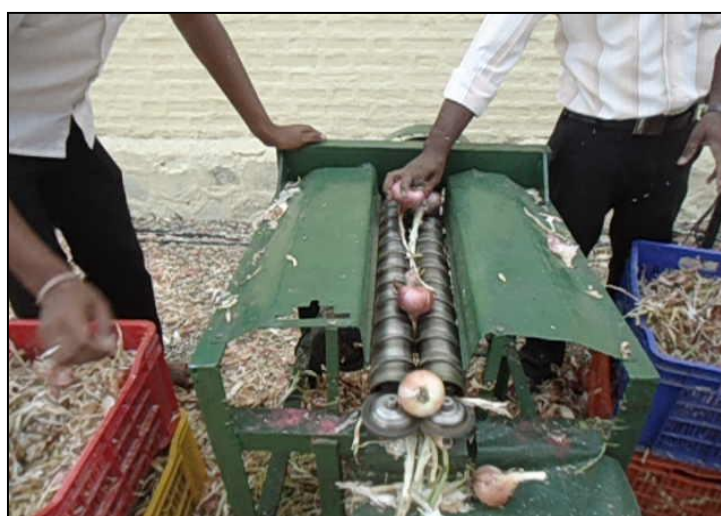
Fig. 7. Power-operated onion de-topper in operation (Bhanage, 2012)
