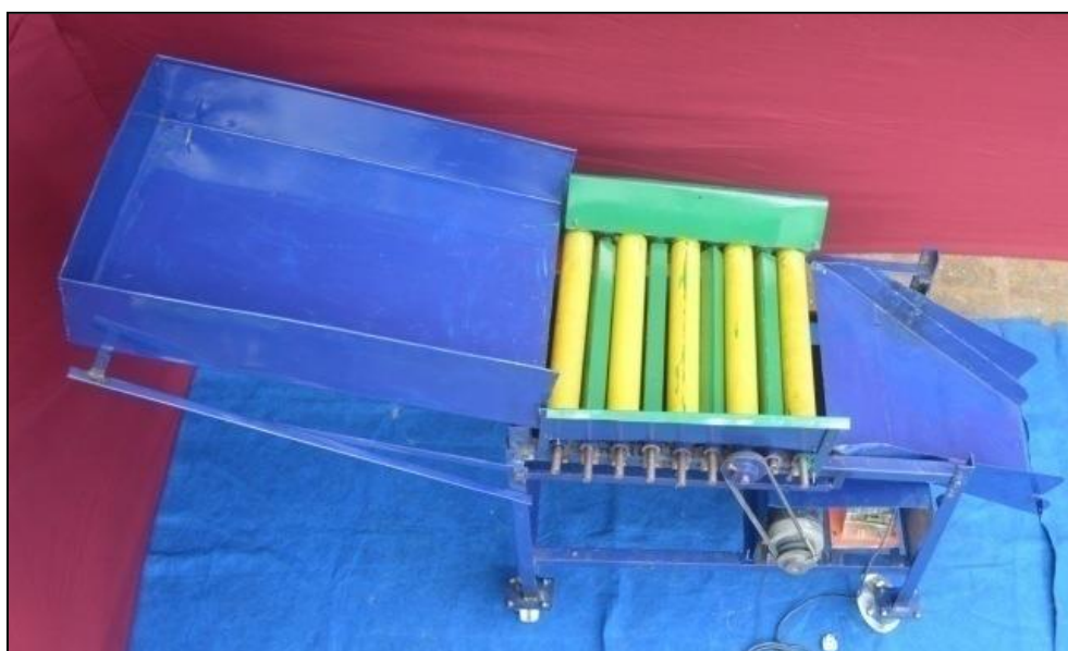
Fig. 9. Power operated onion de-topper (Chittappa, 2016)
