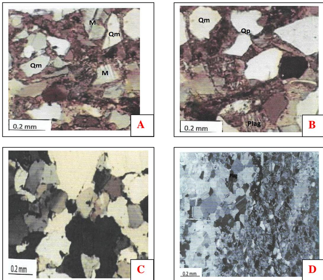
**Fig. 3.** Thin section photographs of sandstones from Eze-Aku Formation (A) Mono-crystalline quartz (Qm) and microcline grain (M), (B) Mono-crystalline quartz - Qm, Polycrystalline quartz grain- Qp and Plagioclase-P) (C) Sub-angular to sub-rounded grains (D) Framework grains bounded by cement
