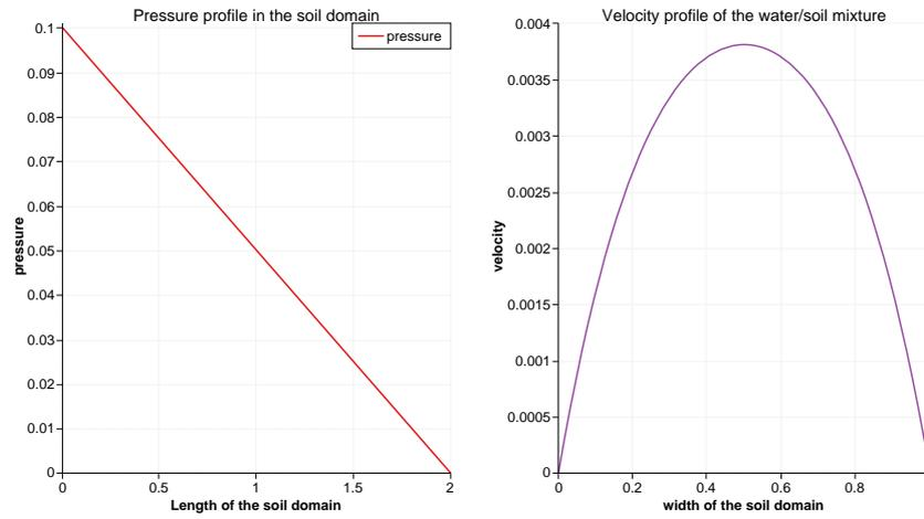
Fig. 3. (a) A snapshot of the Pressure profile in the soil domain (b) Velocity profile in the soil domain
