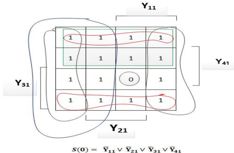
$$S(0) = \bar{Y}_{11} \vee \bar{Y}_{21} \vee \bar{Y}_{31} \vee \bar{Y}_{41}$$
