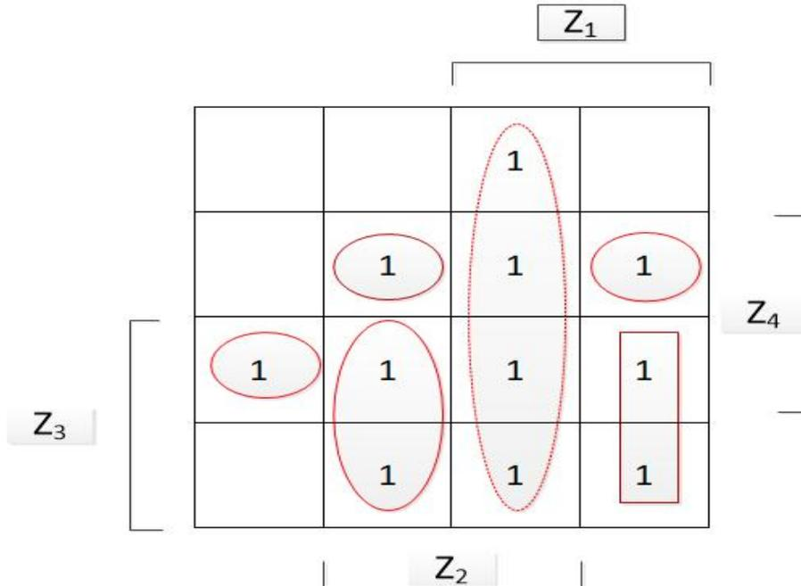
$$(b) \text{Sy}(\{2, 3, 4\}; Z) = Z_1 Z_2 \vee Z_1 \bar{Z}_2 Z_3 \vee Z_1 \bar{Z}_2 \bar{Z}_3 Z_4 \vee \bar{Z}_1 Z_2 Z_3 \vee \bar{Z}_1 Z_2 \bar{Z}_3 Z_4 \vee \bar{Z}_1 \bar{Z}_2 Z_3 Z_4$$
