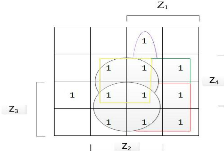
$$(a) \text{Sy}(\{2, 3, 4\}; \mathbf{Z}) = Z_1 Z_2 \vee Z_1 Z_3 \vee Z_1 Z_4 \vee Z_2 Z_3 \vee Z_2 Z_4 \vee Z_3 Z_4$$
