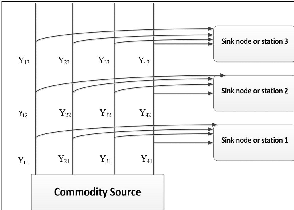
Fig. 1. A commodity-supply system that is modeled as a multi-state k-out-of-n: G system (Adapted from Tian et al. [19]). Here  $Y_{ij}$  denotes the success of section  $j$  of pipeline  $i$  ( $1 \leq i \leq 4$ ,  $1 \leq j \leq 3$ ).
