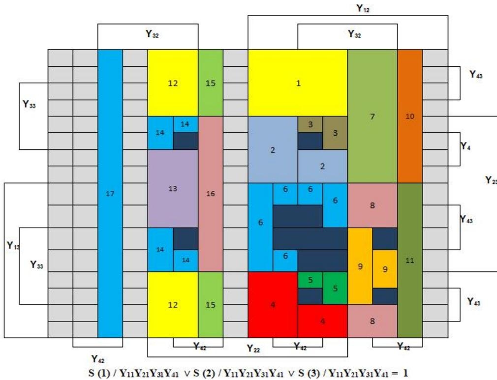
**Fig. 8.** An 8-variable Karnaugh map verifying the identity (38) . Asserted cells for  $S(1) / Y_{11} Y_{21} Y_{31} Y_{41}$  ( Fig. 6 ) are shaded in light grey and those for  $S(3) / Y_{11} Y_{21} Y_{31} Y_{41}$  are marked in dark blue. Other colors in the map label loops for the 17 entries in Table 4, each identified by its assigned integer in Table 4.
