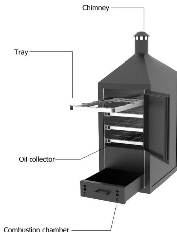
Figure 1. The fish smoke-drying kiln prototype
