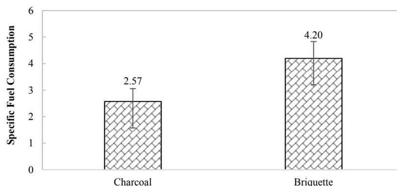
Figure 5. Specific fuel consumption for charcoal and briquette
