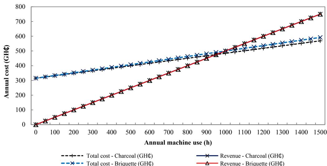
Figure 7. Breakeven chart for the smoke-drying kiln
