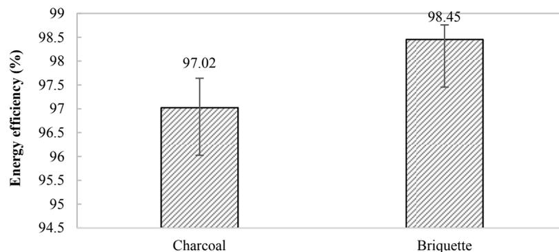
Figure 4. Energy efficiency of the kiln for charcoal and briquette
