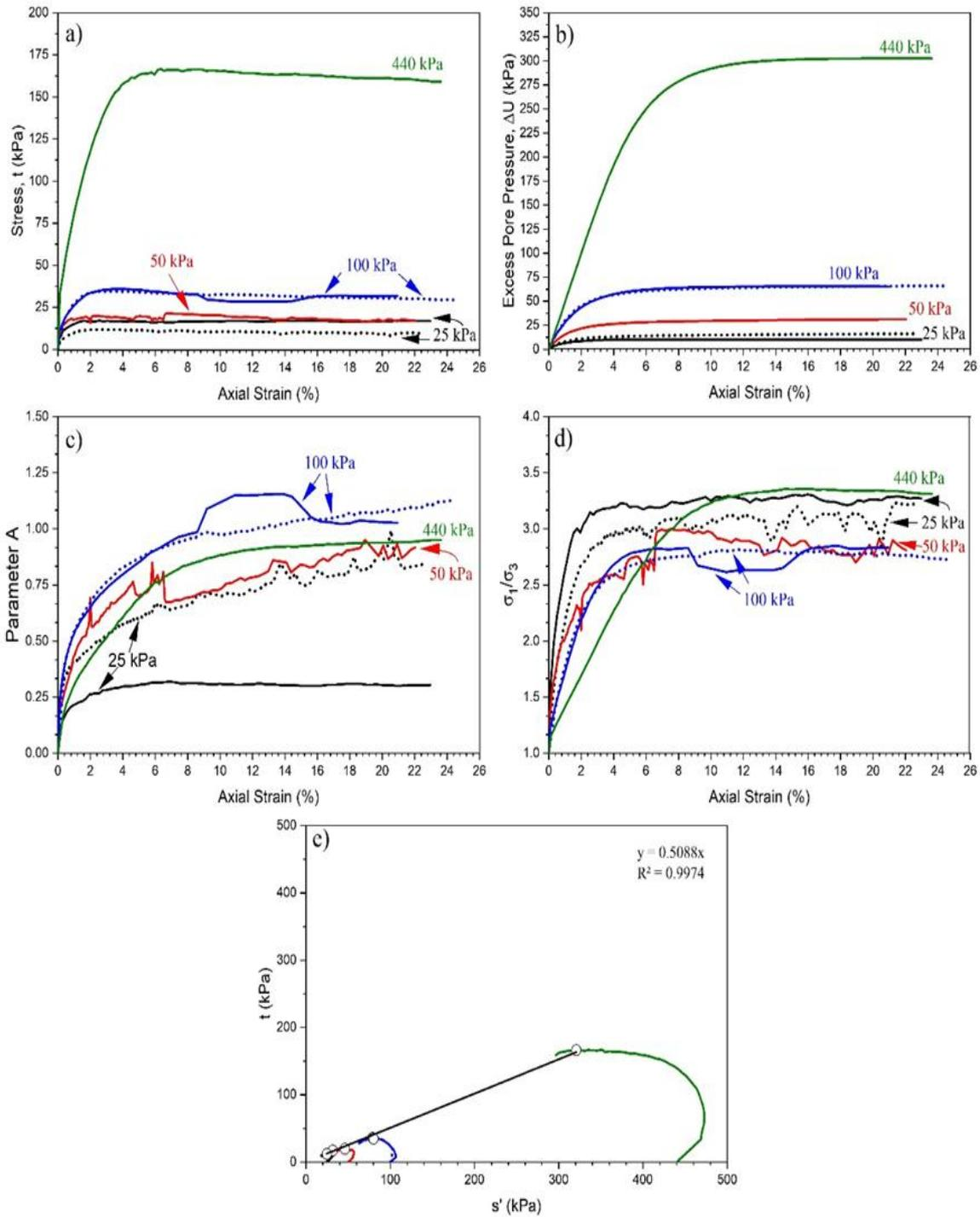
**Fig. 4.** CIU Point 2 (a) Stress,  $t$  (kPa) x Axial Strain (%), (b) Excess Pore Pressure (kPa) x Axial strain (%), (c) Parameter A x Axial Strain (%), (d) Analyse  $\sigma_1/\sigma_3$  (kPa) x Axial Strain (%) and (e) Mohr's wrap in the point 2. The applied stresses of 25, 50, 100 and 440 kPa are represented by black, red, blue and green, respectively. The solid line represents non-percolated samples and the dotted line percolated samples
