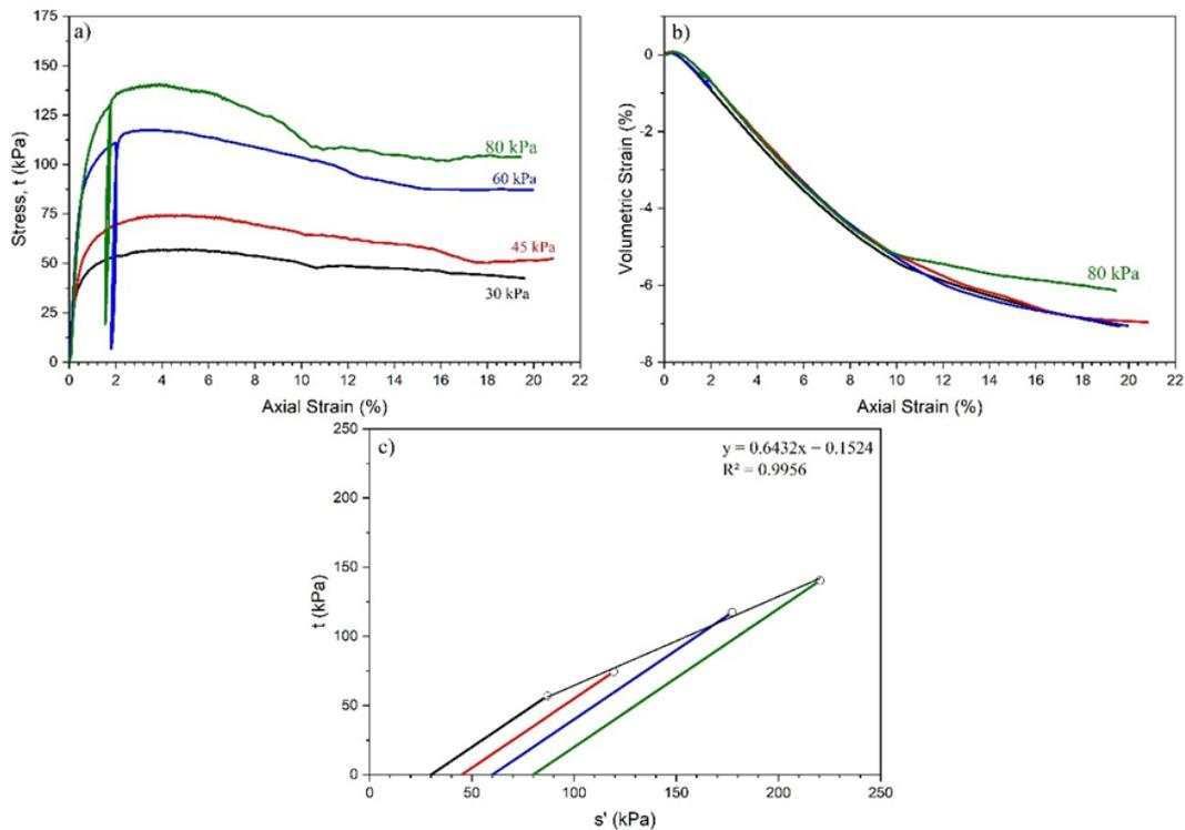
**Fig. 6. CID Point 2 (a) Stress,  $t$  (kPa) x Axial Strain (%), (b) Volumetric Strain (%) x Axial strain (%), (c)  $t$  (kPa) x  $s'$  (kPa), The applied stresses of 30, 45, 60 and 80 kPa are represented by black, red, blue and green, respectively**
