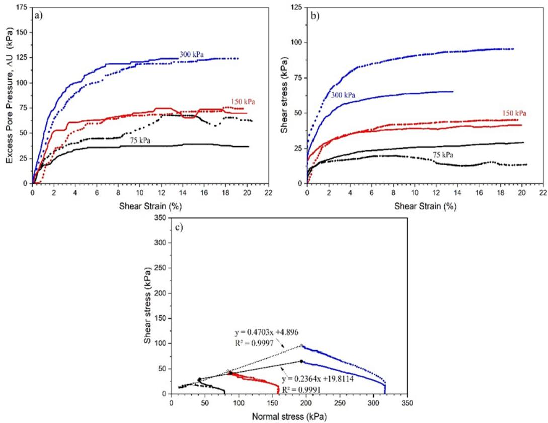
**Fig. 2. (a) Excess Pore Pressure (kPa) x Shear strain (%), (b) Shear Stress (kPa) x Shear Strain (%), (c) Shear Stress (kPa) x Normal Stress (kPa) and Mohr’s wrap in the point 1 (dotted line) and 2 (solid line). The applied stresses of 75, 150 and 300 kPa are represented by black, red and blue, respectively**
