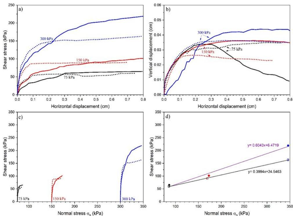
**Fig. 1. (a) Shear Stress (kPa) x Horizontal Displacement (cm), (b) Vertical Displacement (cm) x Horizontal Displacement (cm), (c) Shear Stress (kPa) x Normal Stress (kPa) and (d) Mohr's wrap in the point 1 (dotted line) and 2 (solid line). The applied stresses of 75, 150 and 300 kPa are represented by black, red and blue, respectively**
