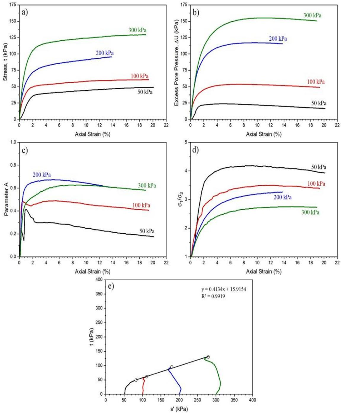
**Fig. 3. CIU Point 1 (a) Stress,  $t$  (kPa) x Axial Strain (%), (b) Excess Pore Pressure (kPa) x Axial strain (%), (c) Parameter A x Axial Strain (%), (d) Analyse  $\sigma_1/\sigma_3$  (kPa) x Axial Strain (%) and (e) Mohr's wrap in the point 1. The applied stresses of 50, 100, 200 and 300 kPa are represented by black, red, blue and green respectively**
