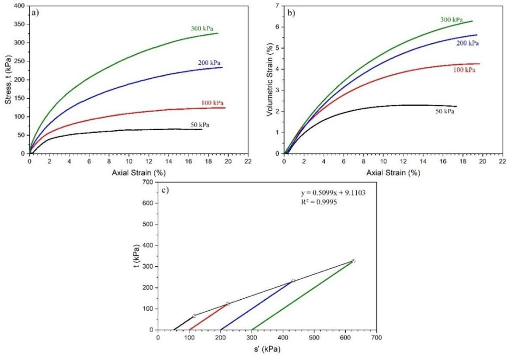
**Fig. 5. CID Point 1 (a) Stress,  $t$  (kPa) x Axial Strain (%), (b) Volumetric Strain (%) x Axial strain (%), (c)  $t$  (kPa) x  $s'$  (kPa), The applied stresses of 50, 100, 200 and 300 are represented by black, red, blue and green, respectively**
