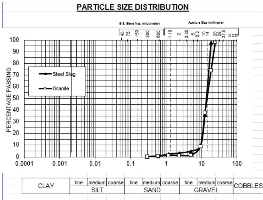
Figure 2. Particle size distribution curve for granite and steel slag
