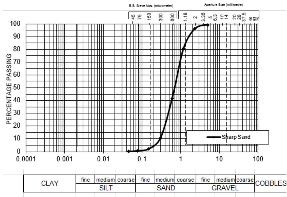
**Figure 1.** Particle size distribution curve for sand
