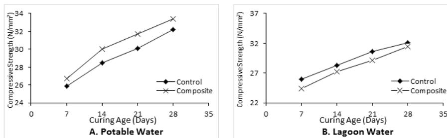
Figure 4. Variation of compressive strength of pozzolan blended steel slag aggregate concrete
