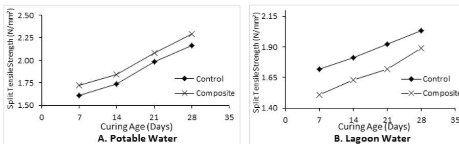
Figure 5. Variation of splitting tensile strength of pozzolan blended steel slag aggregate concrete
