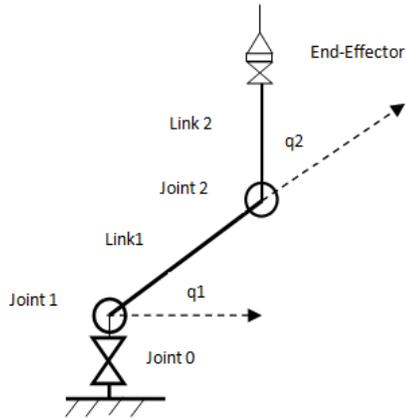
Fig. 4. Kinematics of a two-link 3DOF planar arm
