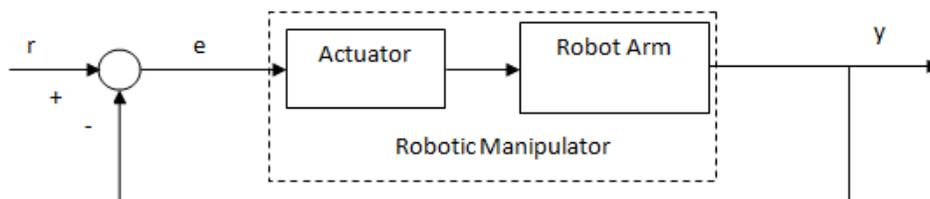
**Fig. 2. Robotic manipulator block diagram (SISO)**
