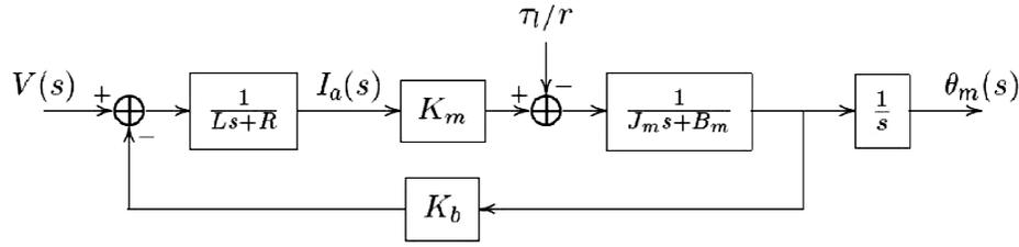
Fig. 3. Block diagram of actuator model with link [14,26]
